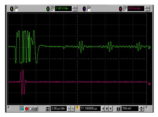
By adjusting the low frequency cut-off knob, the first echo is recovered, as shown in the figure below.
